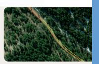
Shoulders are delivered as two features represented as a polygon encompassing 2ft from the edge of travel plus 3ft beyond. A new polygon will be started when the slope changes by more than 1% or if 1/10th of a mile is reached.
